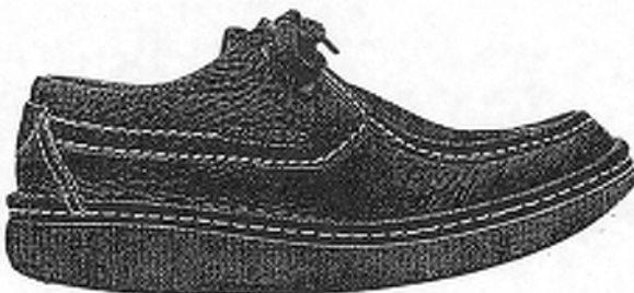
Fig. 12: Toe spring, the uptilt of toe end of the shoe; built into the last and transferred to the shoe.
